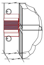
If interference between the two seal flaps occurs, remove one of the flaps by peeling it off.
