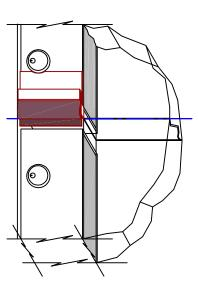
If a substantial portion of the seal's mounting plate was removed to eliminate interferences, use the two self-tapping mounting screws provided for a more secure mounting.
